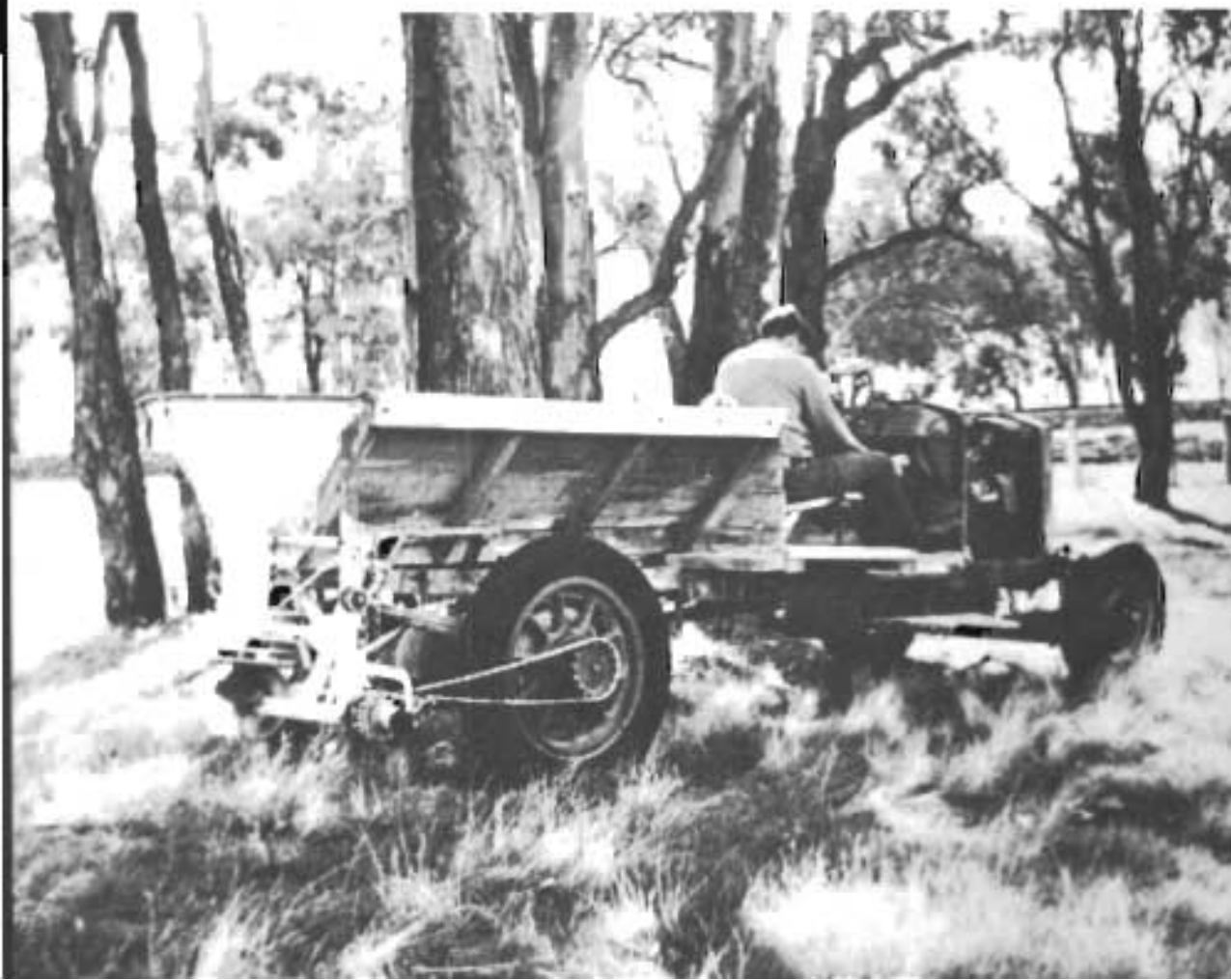
Early "spinner" type fertiliser spreader mounted on a motor vehicle chassis.
