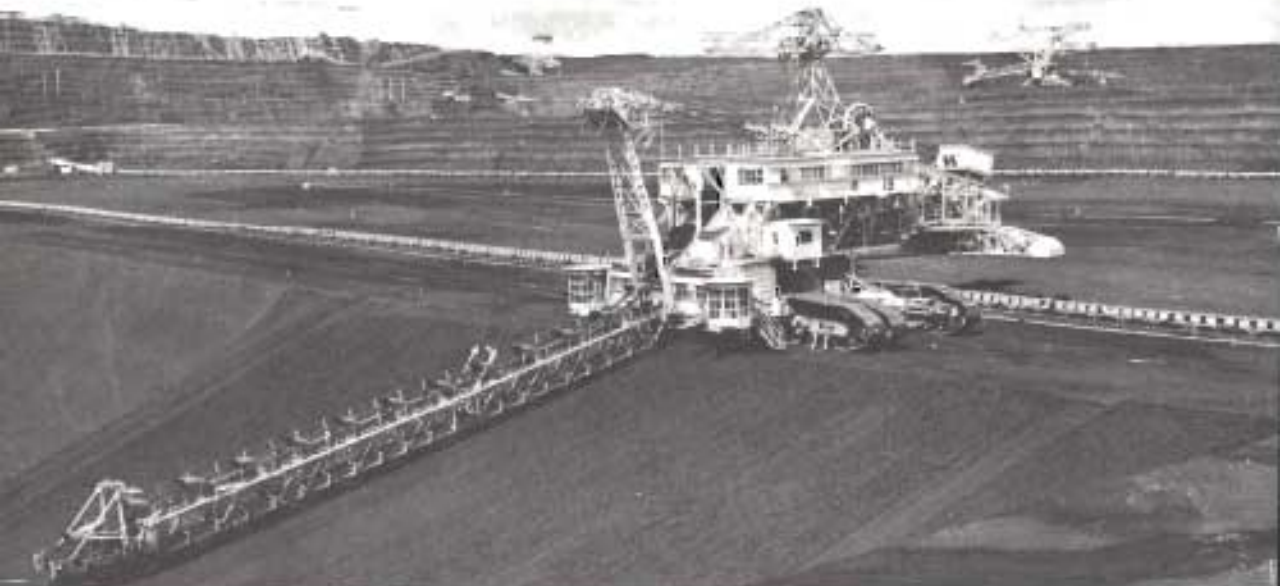
Bucket-chain dredge at the Morwell brown coal open cut State Electricity Commission
