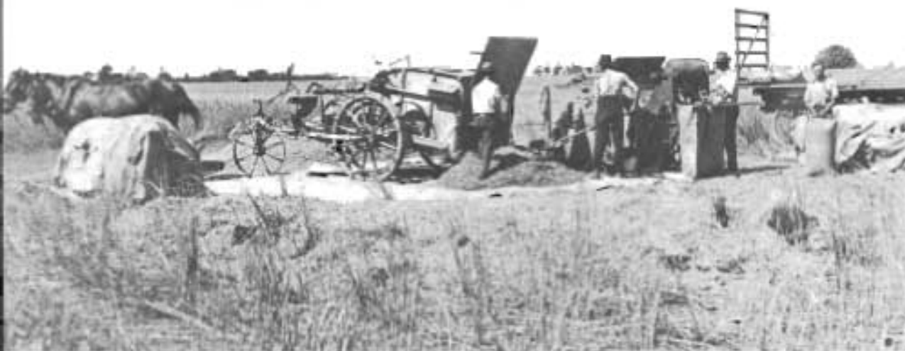
Stripper and winnower, early grain harvesting machinery.
